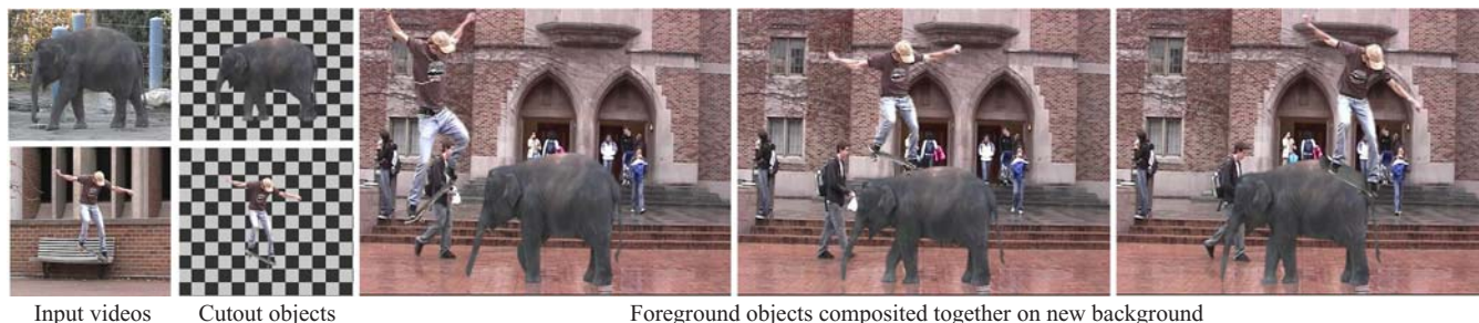
Figure 1: Our interactive video cutout system makes it easy to extract the foreground objects in these videos of an elephant and a skateboarder. We then composite these objects onto a third background video to form a new video in which the skateboarder skates on the elephant.
